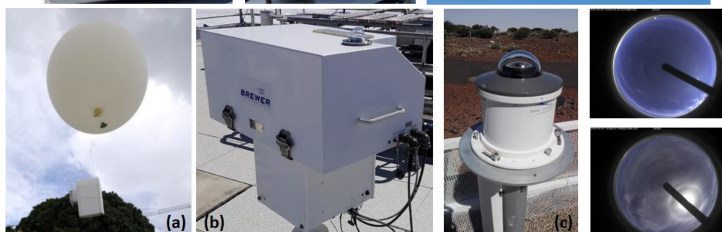
Figure 4. Other instruments currently used at IZA BSRN (a) radiosonde profiles, (b) Brewer spectrophotometer and (c) All-Sky SONA camera (Automatic Cloud Observation System) installed at IZA and images taken by the camera.
