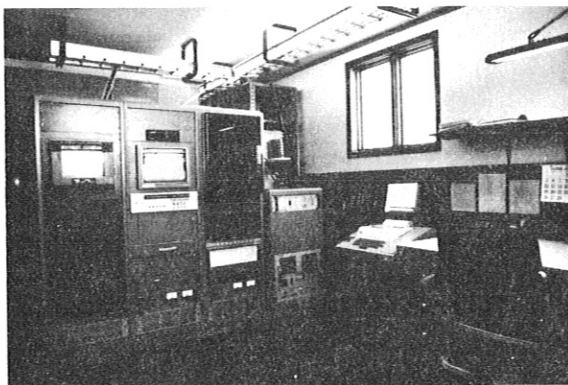
Figure 59. ICDAS and associated electronics in the Clean Air Facility at the Amundsen-Scott Station, South Pole, Antarctica.
