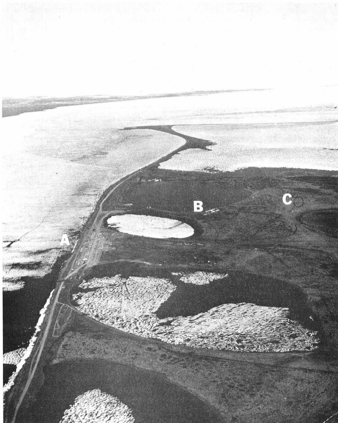
Figure 1. Point Barrow complex in 1971. A - Naval Arctic Research Laboratories. B - POW-Main DEW Station (USAF). C - Location of GMCC Observatory (constructed in 1972).
