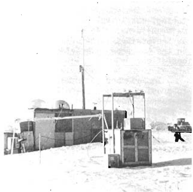
Figure 1. Temporary solar radiation platform with the Aurora Tower and the aerosol/gas sampling mast in the background.
