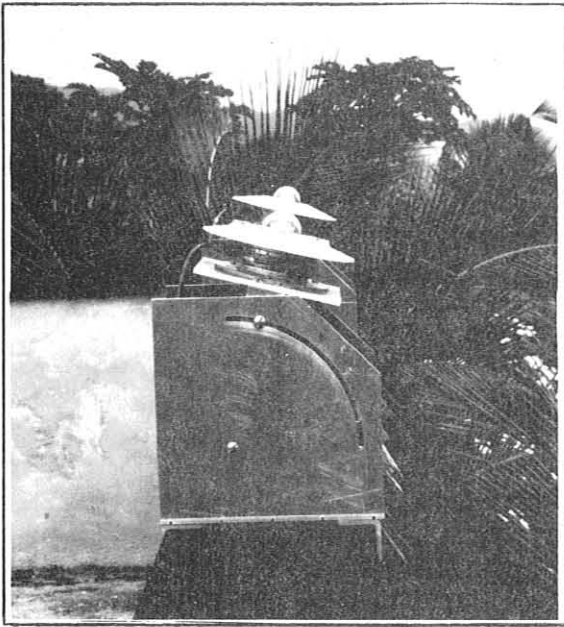
Figure 56.--Pyranometers on tilted stands on the roof of the SMO observatory.
