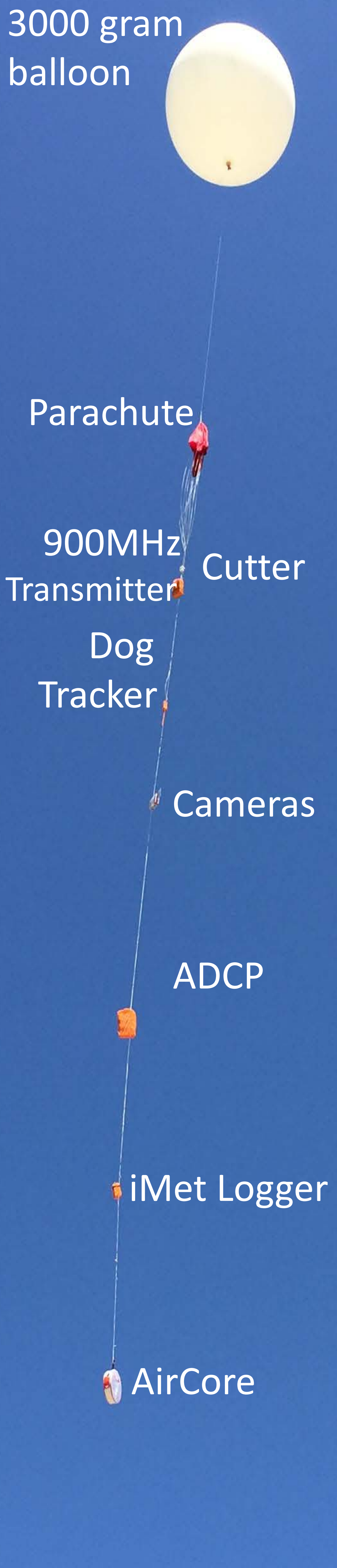
Current AirCore design, with a 100 m 1/8" SS tubing coil.
