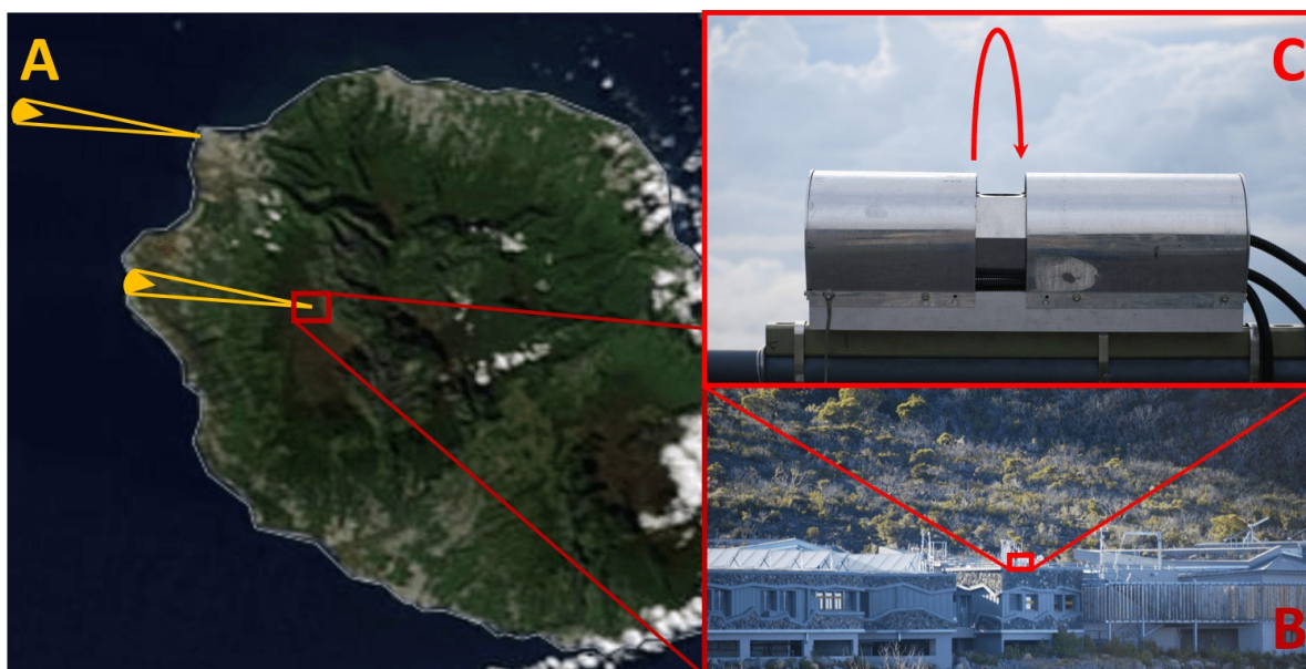
Figure 1. A) MODIS imagery of La Réunion Island in the southwest Indian Ocean from June 11, 2017. Arcs indicate the viewing direction of the Royal Belgian Institute for Space Aeronomy (BIRA) operated MAX-DOAS in Le Port on the coast and the CU-Boulder MAX-DOAS at Maïdo Observatory at 2.16 km. B) The Maïdo Observatory. The MAX-DOAS telescope is mounted on the roof with the rest of the instrument below it. During the intensive phase other instruments will be on the roof, or use inlets extending above the roof, or horizontally from the observatory. C) The CU-Boulder MAX-DOAS telescope. The telescope can move in the vertical plane perpendicular to photo to gather profile information by probing different altitudes.
