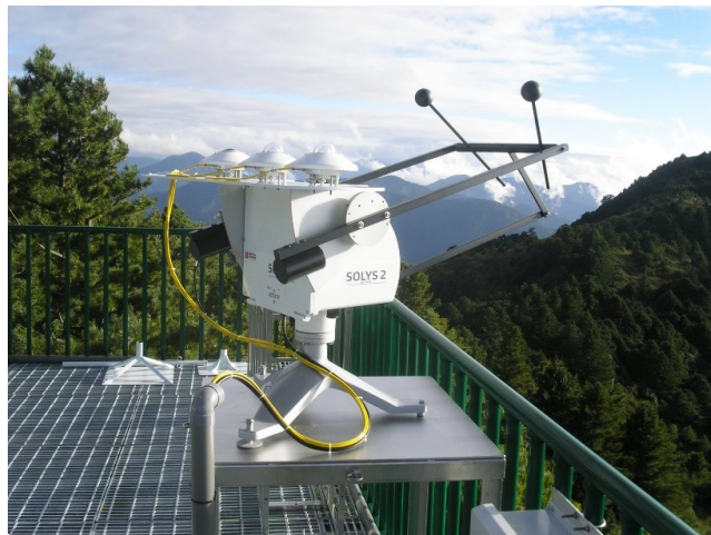
Figure 2. Sun tracker and radiometers used at Lulin station.
