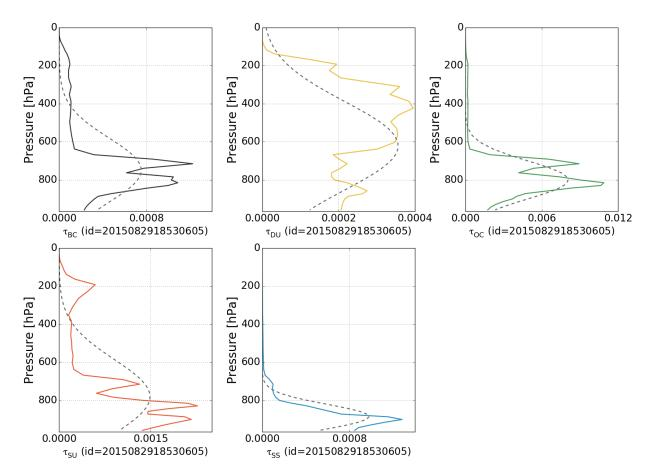
**Figure 1.** Example of fitting Gaussians to the GEOS-5 aerosol profiles in order to ingest them into the OCO-2 retrieval algorithm.
