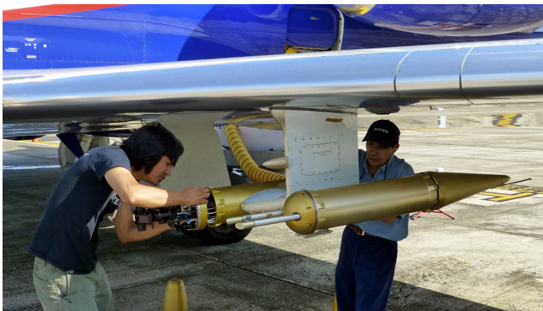
Figure 1. The University of Colorado Airborne MAX-DOAS instrument telescope mounted below the wing of the NSF/NCAR GV aircraft is being serviced by CU graduate student Sunil Baidar. The instrument measured sub-pptv concentrations of BrO and IO radicals directly in the open atmosphere, spanning altitudes from the tropical Marine Boundary Layer (MBL) into the tropical transition layer (TTL), and the sub-tropical lower stratosphere (LS) during the TORERO and CONTRAST field campaigns.
