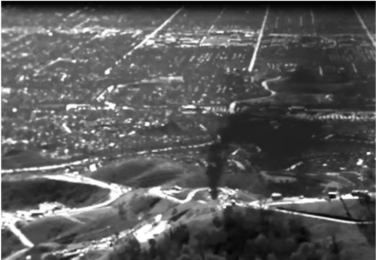
Figure 1. IR camera image of leaking \text{CH}_4 plume from Aliso Canyon well SS-25. Image courtesy of Environmental Defense Fund.
