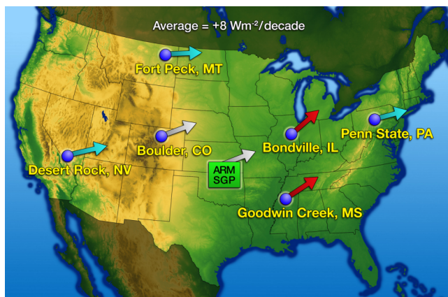
Figure 1. Graphic illustration of overall relative surface downwelling all-sky shortwave brightening trends at the U.S. SURFRAD and ARM sites from 1996 through 2007 (Long et al., 2009).
