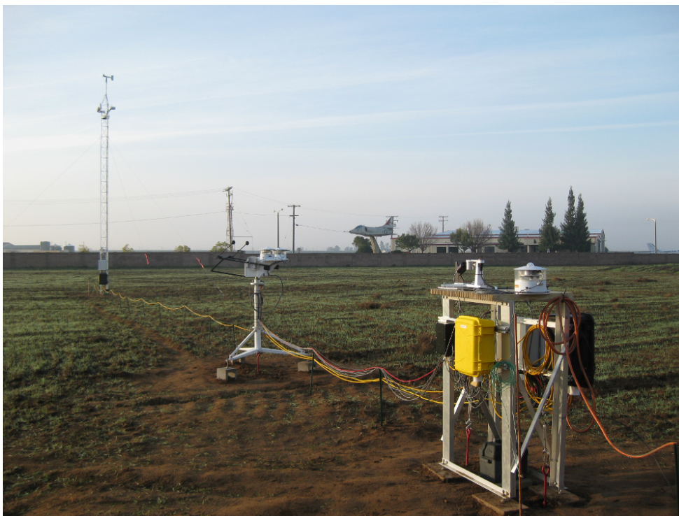
Figure 1. Mobile SURFRAD suite of instrumentation at the DISCOVER-AQ Campaign in the San Joaquin Valley, CA.
