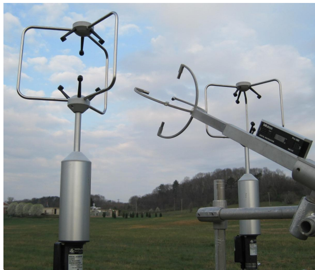
Figure 2. Photograph of the Applied Technologies sensor (center) tilted 30° during the experiment.
