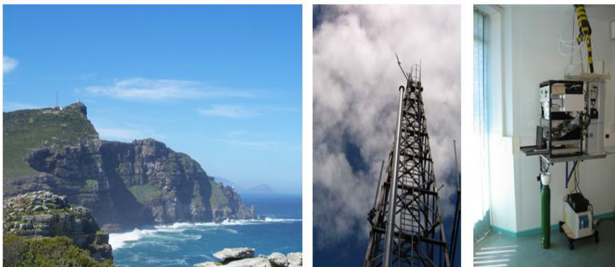
Figure 1. Left : 30m sampling mast in perspective to coastal cliff; Middle : aerosol sampling stack mounted onto mast; Right : sampling system showing PSAP and Nephelometer location inside laboratory.
