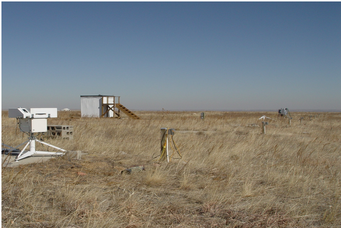
Figure 1. Brewer Spectrophotometer 93-101 operating at the Table Mountain Test Facility, Boulder, Colorado. The Brewer is collocated with the USDA's reference UV spectroradiometer and the State University of New York's UV-rotating shadowband spectroradiometer.
