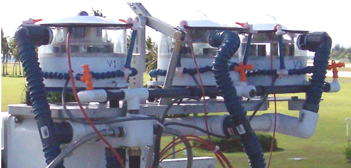
Figure 1. The modified ventilator housings and air manifold components installed during December 2004 at the Kwajalein BSRN site.
