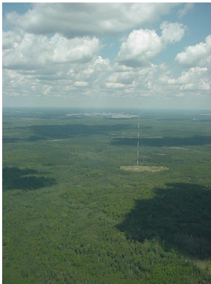
Figure 1. Photo showing a 447-m-tall television transmitter tower in northern Wisconsin, which CMDL uses to measure CO 2 mixing ratios up to 400 m above the ground. The atmospheric boundary layer (ABL) depth is approximated by the cloud base. In this poster we discuss the budget of CO 2 within the ABL.
