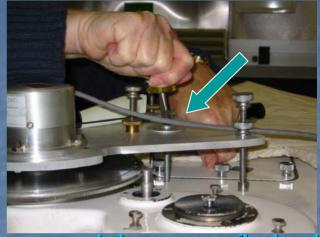
Once set screw is loose, use a flat head screw driver to remove large bolt that attaches the encoder to the Dobson
