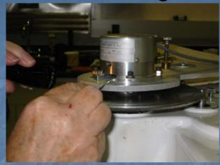
Use Allen wrench to loosen set screw (may be two screws)
