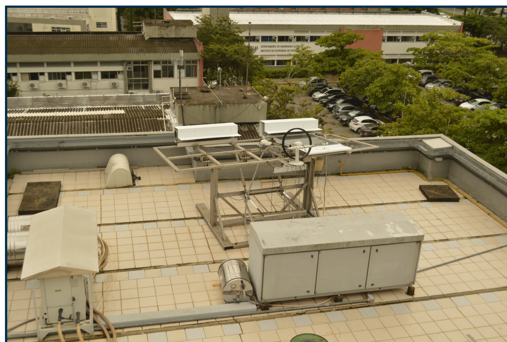
Solar collector test bench and peripheric control units
