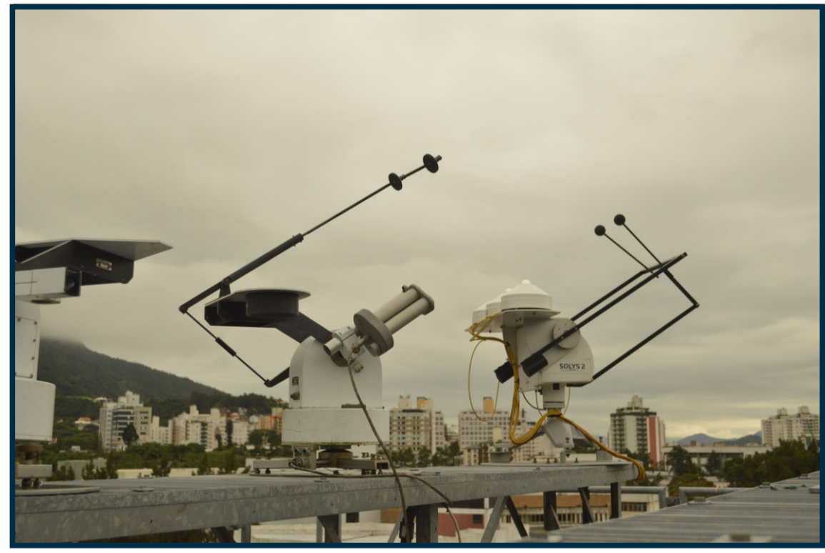
Picture of the three solar trackers, one of them for radiometers calibration
