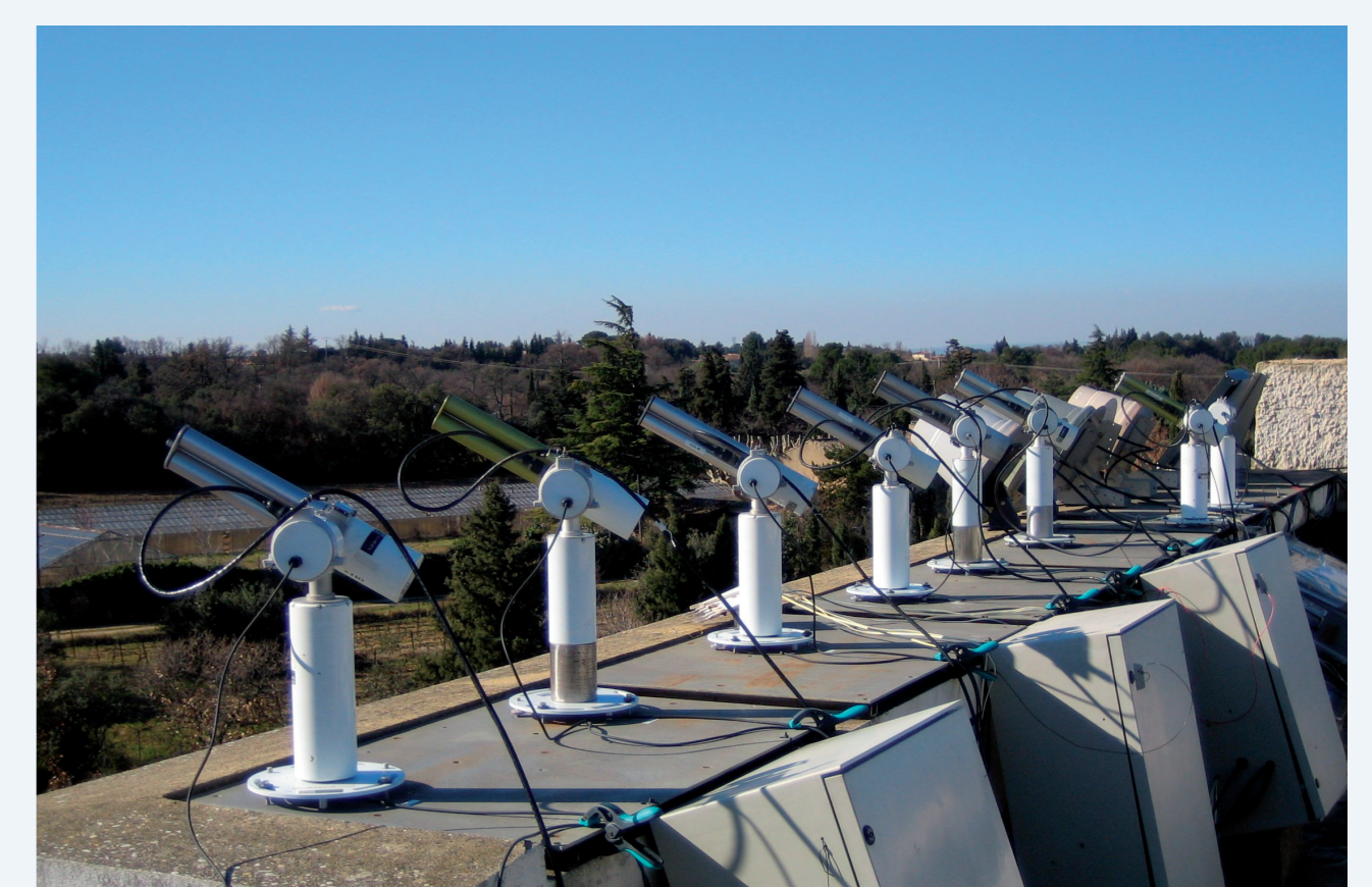
Photometers calibration on the terrace
