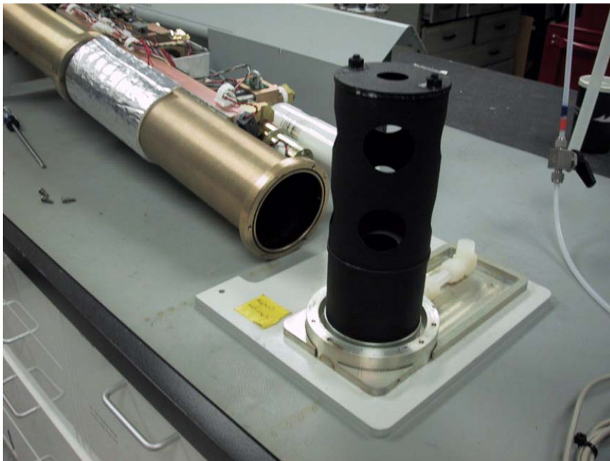
Fig. 16. The nephelometer light trap column.
