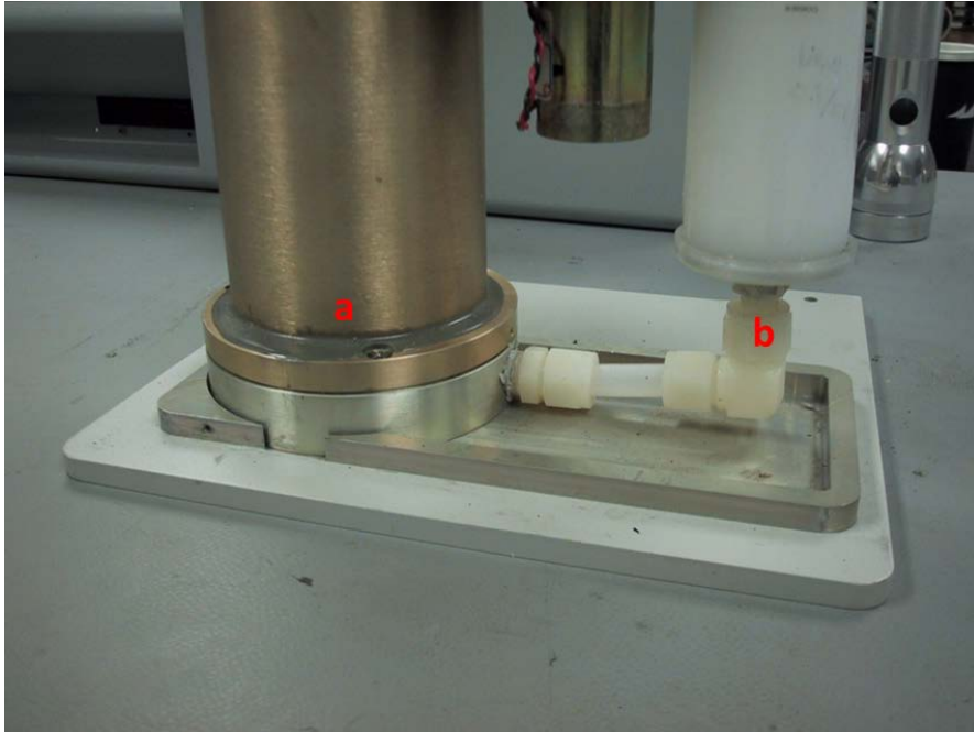
Fig. 15. Removal of the bottom flange for access to the light trap.
