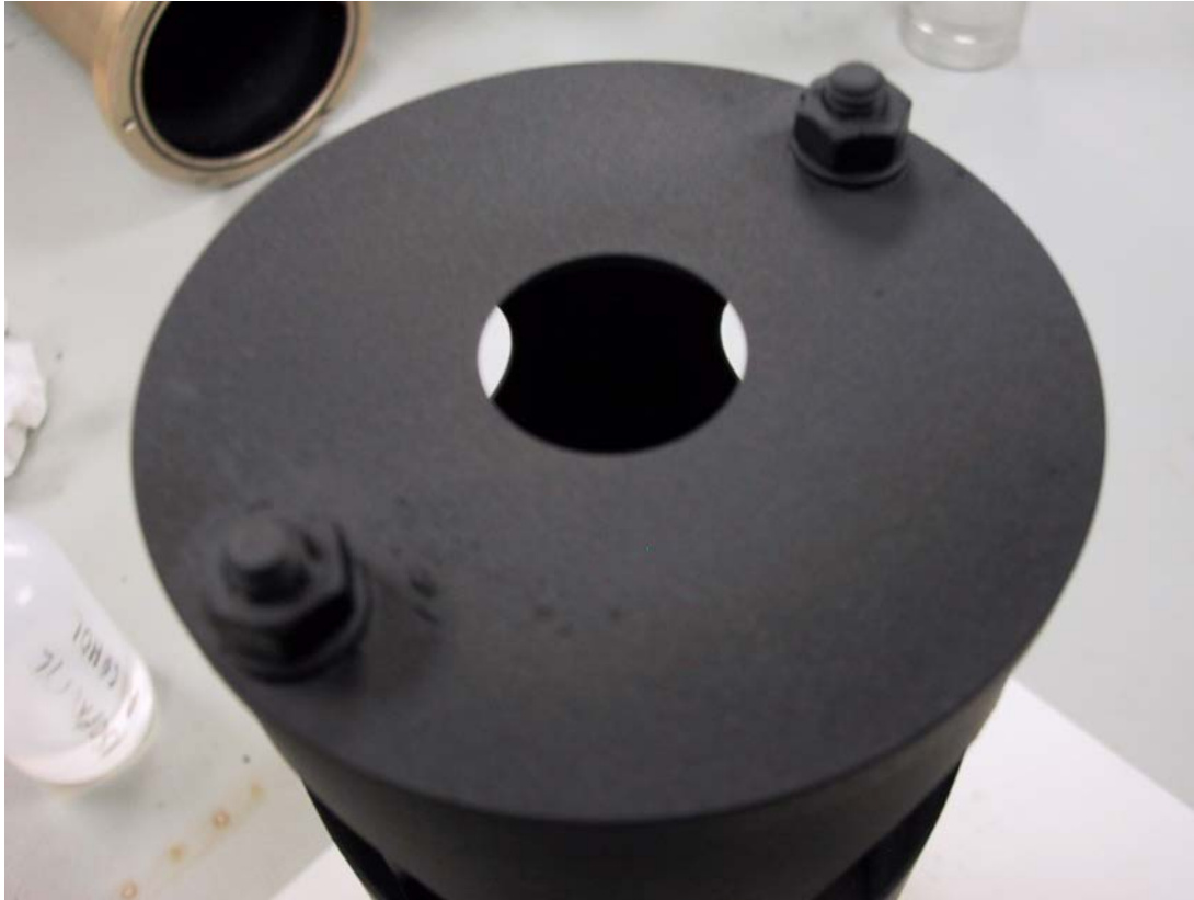
Fig. 17. The first aperture in the light trap column.
