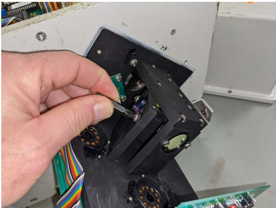
Fig. 11. Securing the color bandpass filter using a small Phillips screwdriver.
