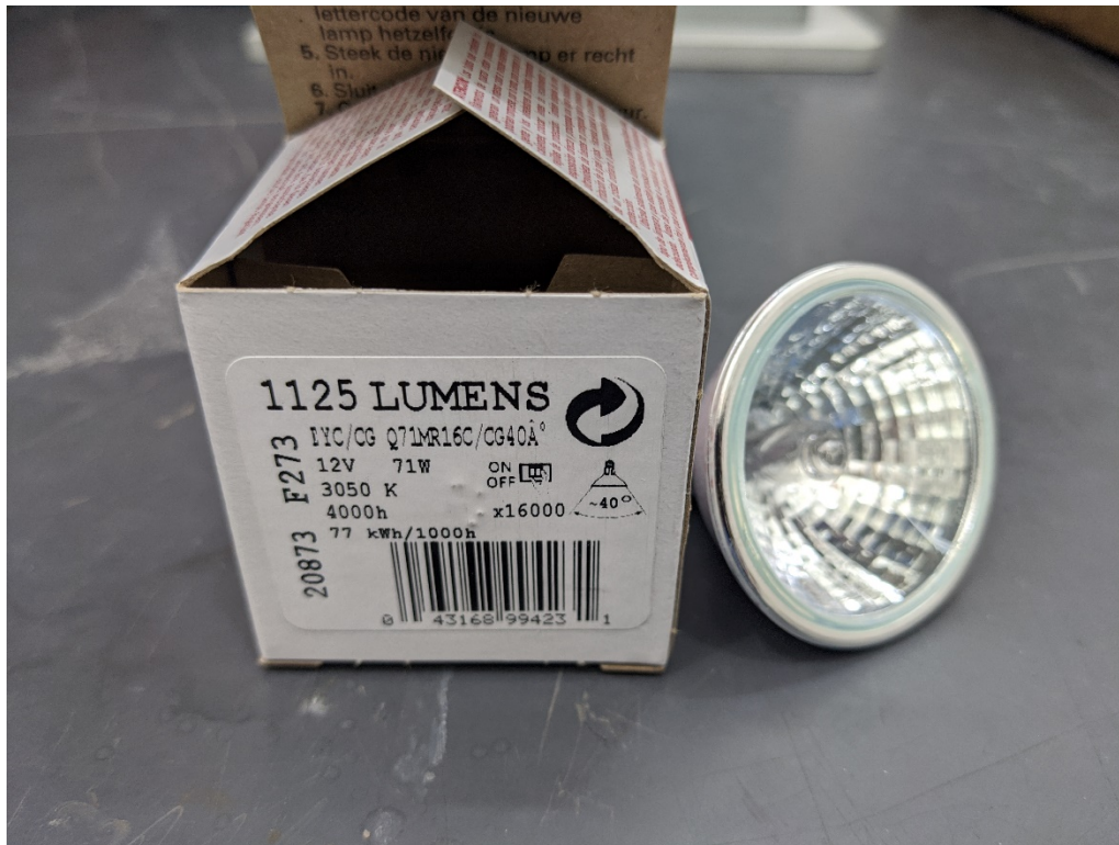
Fig. 2. Nephelometer lamp GE 20873 EYC/CG Q71MR16C/CG40A.
